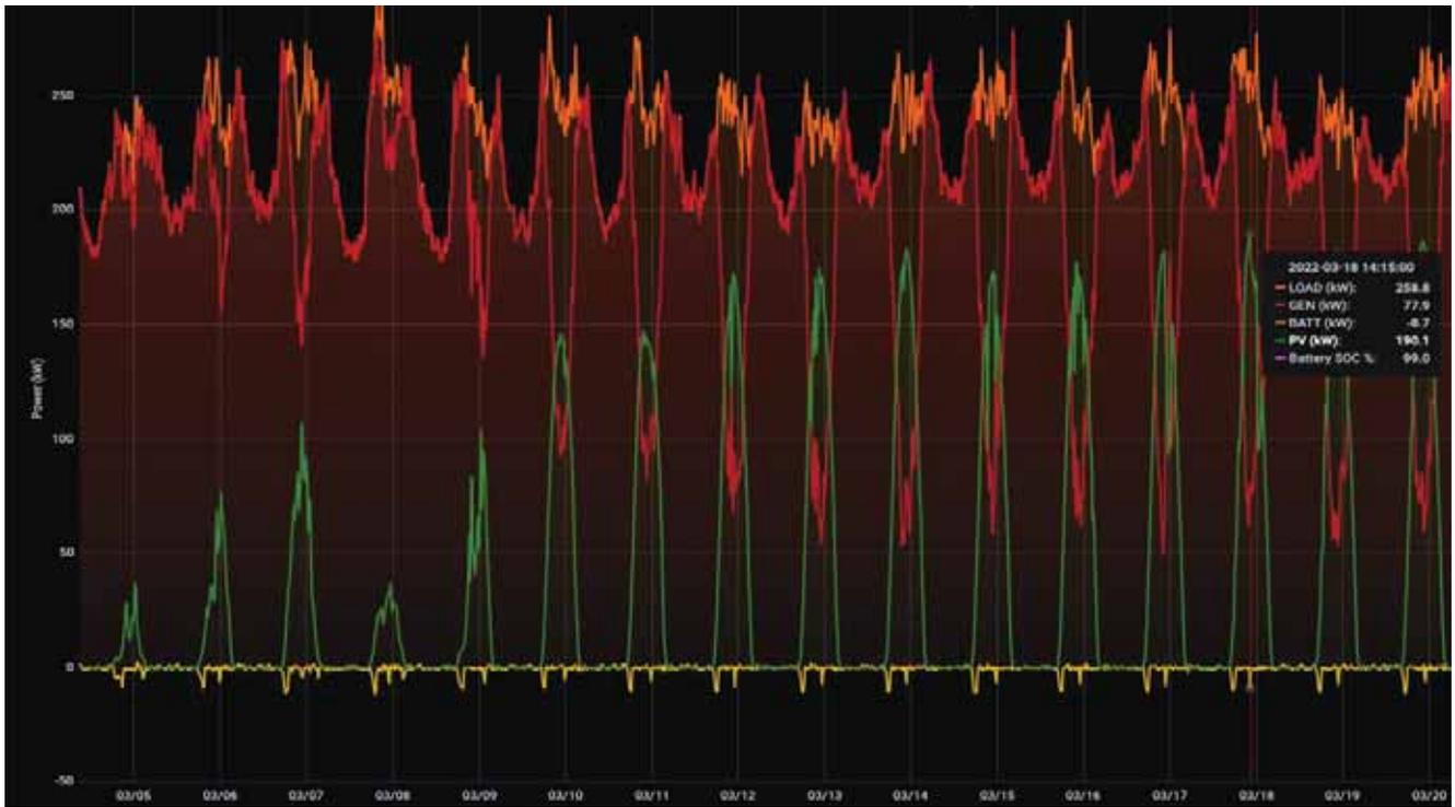
Figure 23. Shungnak Solar Production Over a Two-Week Period in March 2022
