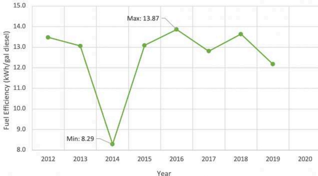
A higher fuel efficiency results in less diesel fuel use and a lower cost to generate power. A fuel efficiency below 12 kWh/gal is poor; a fuel efficiency above 14 kWh/gal is excellent. The fuel efficiency in Deering has typically been very good, but there is some variation year to year. The data for 2014 may be inaccurate as it is exceptionally low. No data was available for 2020.
