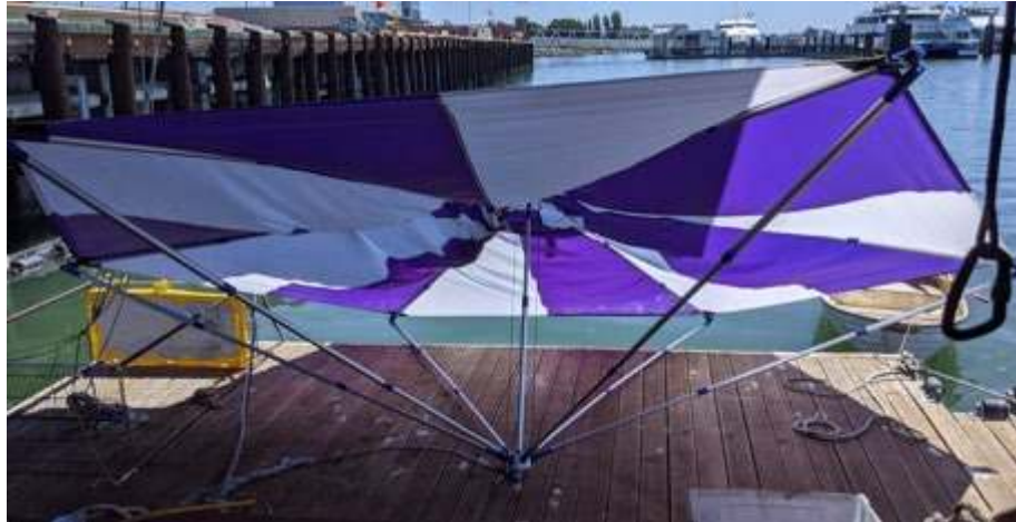
Figure 2. Methane collector “funnels” measure approx. 15 feet
