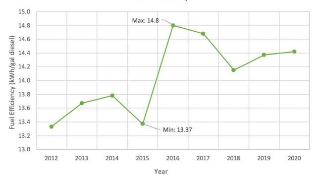
A higher fuel efficiency results in less diesel fuel use and a lower cost to generate power. A fuel efficiency below 12 kWh/gal is poor; a fuel efficiency above 14 kWh/gal is excellent. The fuel efficiency in Kivalina historically has been good. Starting in 2016, there was a distinct improvement in efficiency to values consistently exceeding 14 kWh/gal of diesel. This improvement may correlate with generator upgrades.
