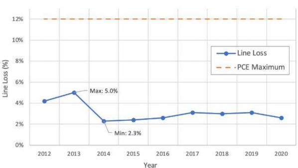
The maximum allowable line loss to maintain eligibility for PCE benefits is 12%. In Kivalina, the line loss is very low and has been very low for the past nine years, indicating the distribution system is in good condition and all power use is accounted for. As more of the village load moves to the new location, it is expected that some additional line loss will occur from the diesel power plant, but this may be offset by new renewable energy generation located closer to the new village loads.
