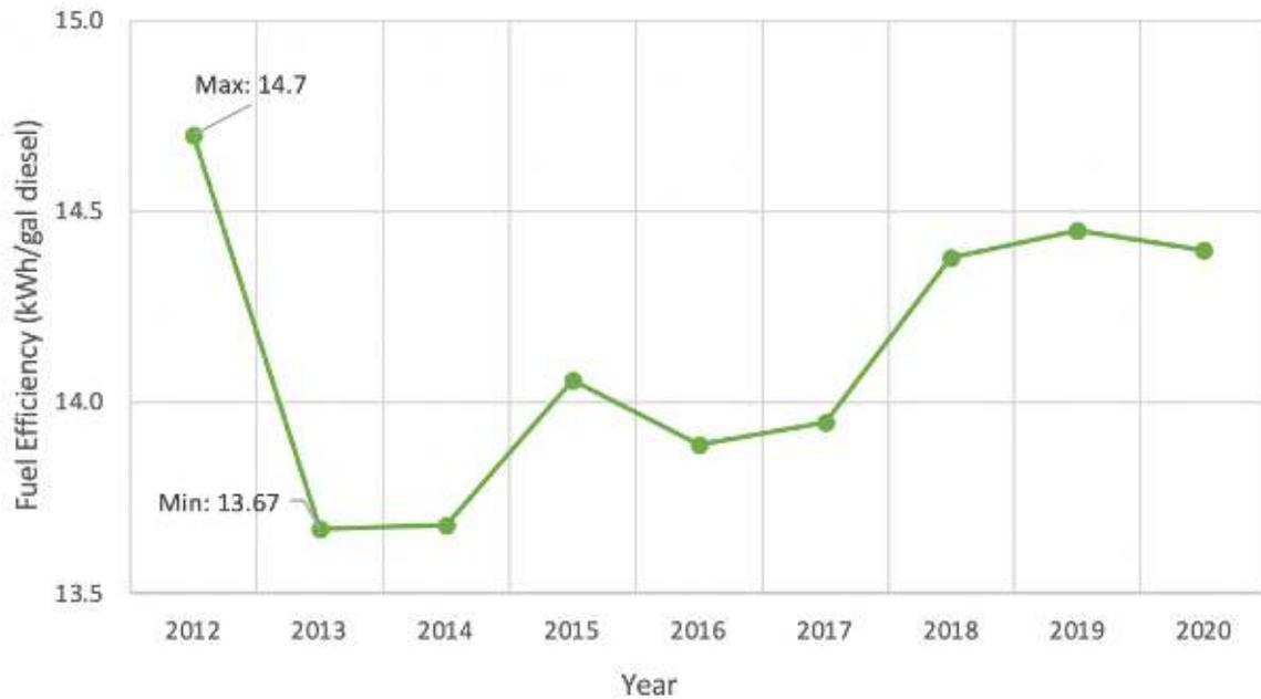
A higher fuel efficiency results in less diesel fuel use and a lower cost to generate power. A fuel efficiency below 12 kWh/gal is poor; a fuel efficiency above 14 kWh/gal is excellent. The fuel efficiency in Kiana is very good, especially since 2018 with fuel efficiencies that are consistently greater than 14 kWh/gal of diesel.
