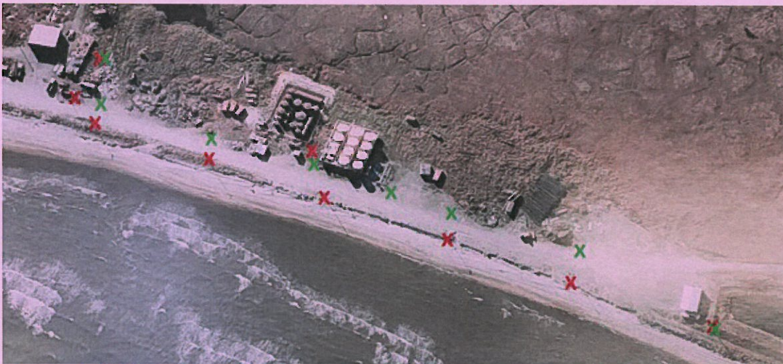
Figure 1. Power poles in Deering. Red X is the old pole locations. Green X is the new pole locations
